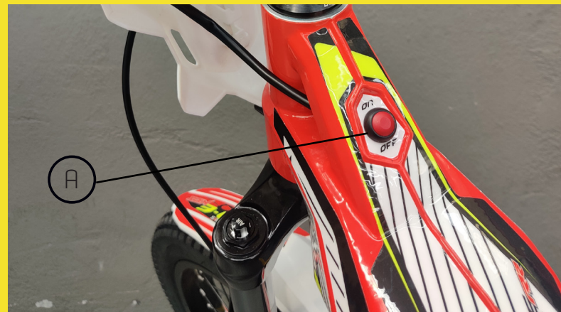
Figure A) Switch ON /OFF locates on the chassis
