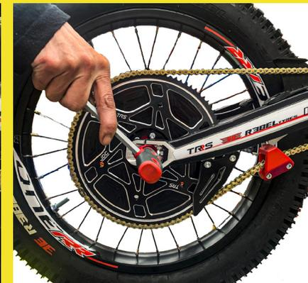
Unscrew the rear wheel axle with a 8mm Allen wrench.
