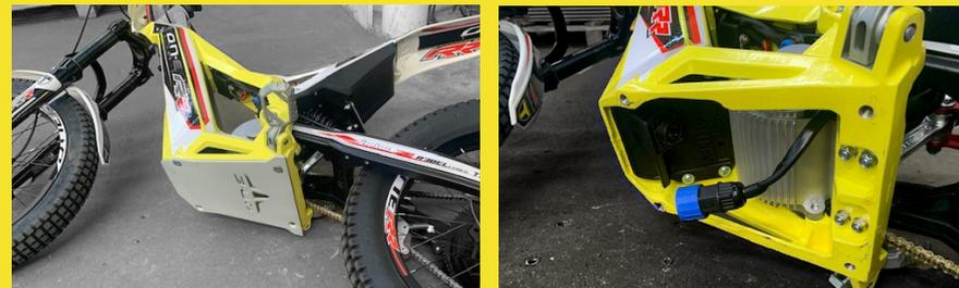
Put your ON-E on the ground and with a 5 mm Allen wrench, remove the 4 screws from skid plate of the chassis and unplug the connector from the battery twisting the lock ring counterclockwise.
