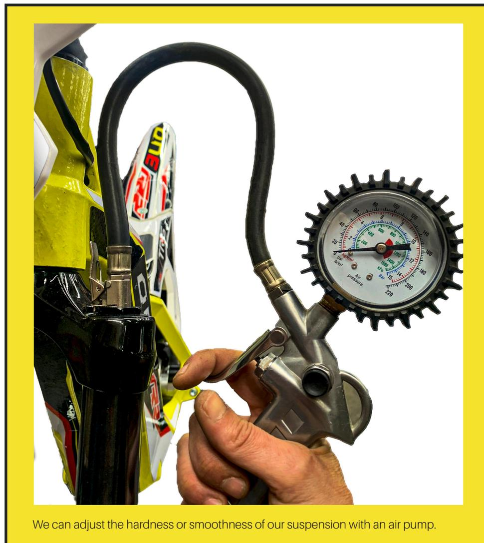
We can adjust the hardness or smoothness of our suspension with an air pump.
