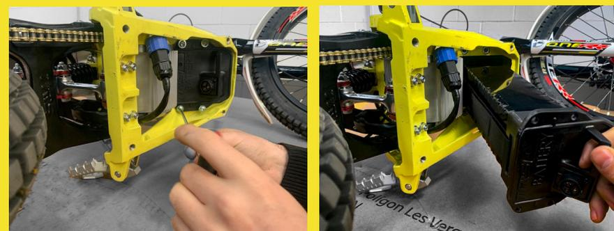
Then remove the screws from the plastic cover battery with a 4mm allen wrench and take off the battery.
