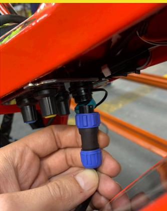
Put in the correct position the two-pin plug (fig F) aligning the white dot with the protrude from the charging connector (fig E). Screwed in the nut that brings the two-pin plug (fig D). Replace the blue cap when the battery is fully charged.
