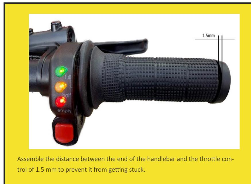
Assemble the distance between the end of the handlebar and the throttle control of 1.5 mm to prevent it from getting stuck.
